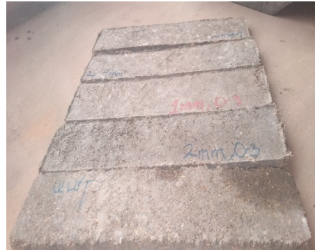
Fig. 5. The fibre cement boards.
