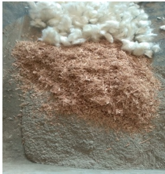
Fig. 4. A mixture of rattan, PVA fibre and cement.
