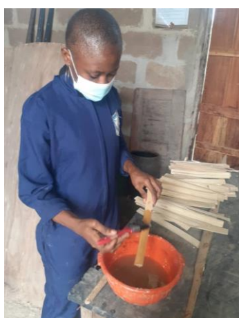
Fig. 12. Coating the strips.
