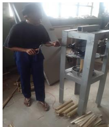
Fig. 8. Splitter being operated with a screw jack.
