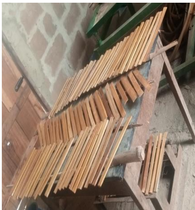
Fig. 14. Air-drying the coated bamboo strips.
