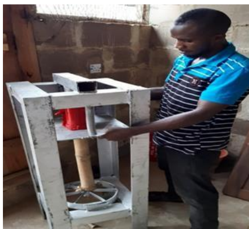
Fig. 7. Splitter being operated with hydraulic jack.
