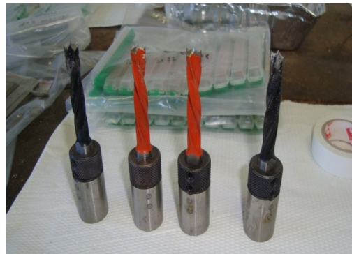
Fig. 2. Burghie elicoidale dublu-spiralate / Twist drills with dual-spirals.
