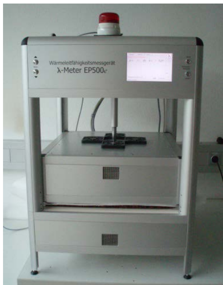
Fig. 4 Measuring device for thermal conductivity (Lambda-Meter EP500).
