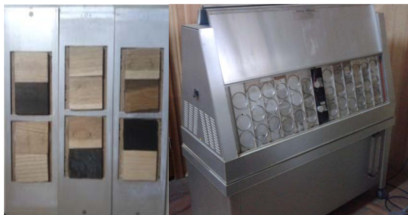
Fig. 1 Weathering test specimens and accelerated weathering tester.
