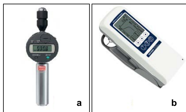
Fig. 2 a - Hardness meter (Mitutoyo Hardmatic-HH-334; b - Colour and gloss meter (Nippon Denshoku-NF999).
