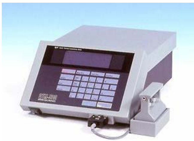
Fig. 1 Quick Thermal Conductivity-500 type device used for thermal conductivity measurements at Karabük University.
