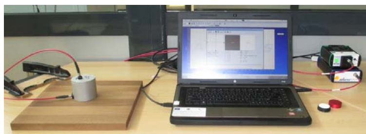
Fig. 3. AVANTES AVA SPEC 2048 spectrophotometer used for the colour stability evaluation of the panels.
