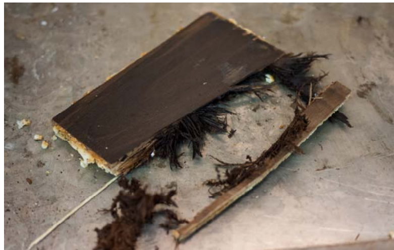
Fig. 4. Exploded panel of specimen group 7. Apparently, the pressing time was too long, or the pressing temperature too high
