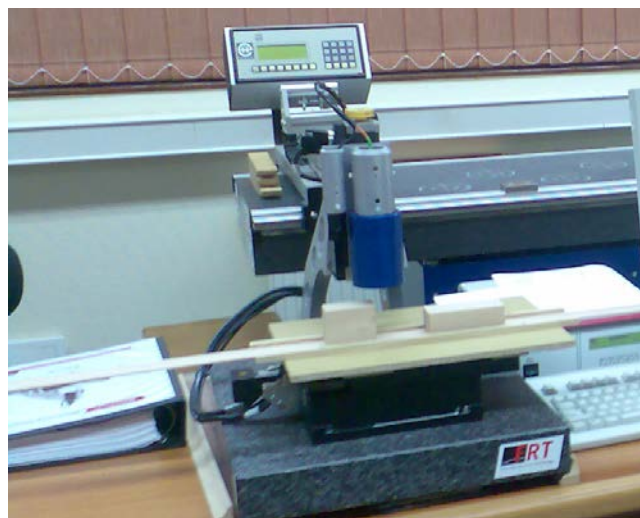
Fig. 4. MicroProf FRT roughness device
