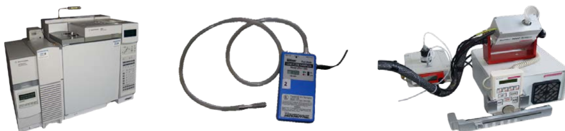
Fig. 2. Equipment for testing VOC emissions
