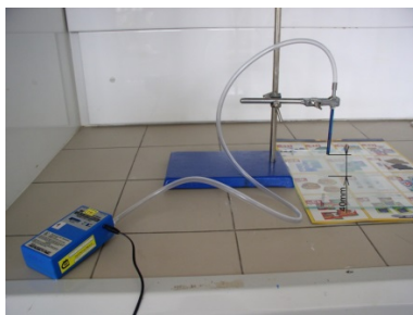
Fig. 1. Equipment for measuring emitted emissions
