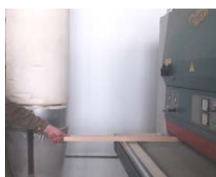
e) calibrating – using the wide tape sanding machine
