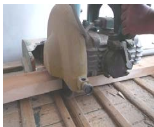
a) cross-cutting – using the circular saw
