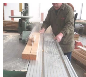
c) ripping – using the circular saw
