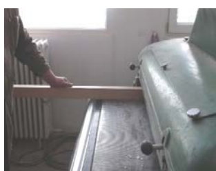
d) planing to final thickness – using the planing machine
