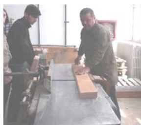
b) edge-face straightening – using the straightening machine
