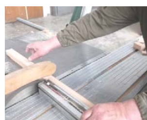
f) cutting to length – using the circular saw
