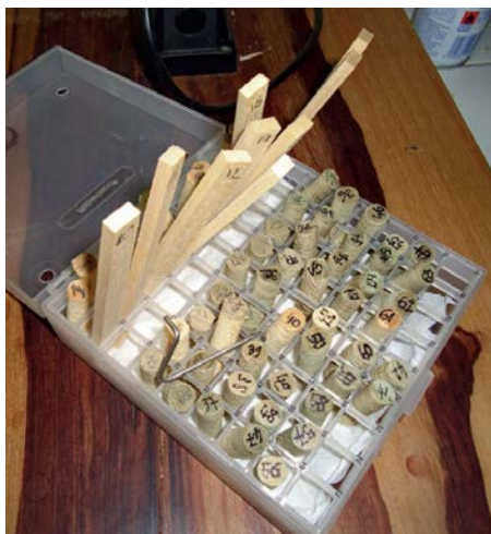
Fig. 1. Samples of woods non treated and treated with PCP and CCA
