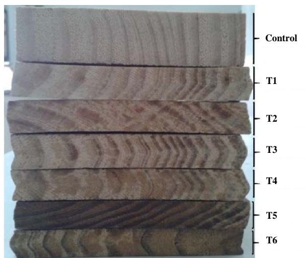
Fig. 2. View of the thickness and the shape of the board after the thermomechanical treatments.
