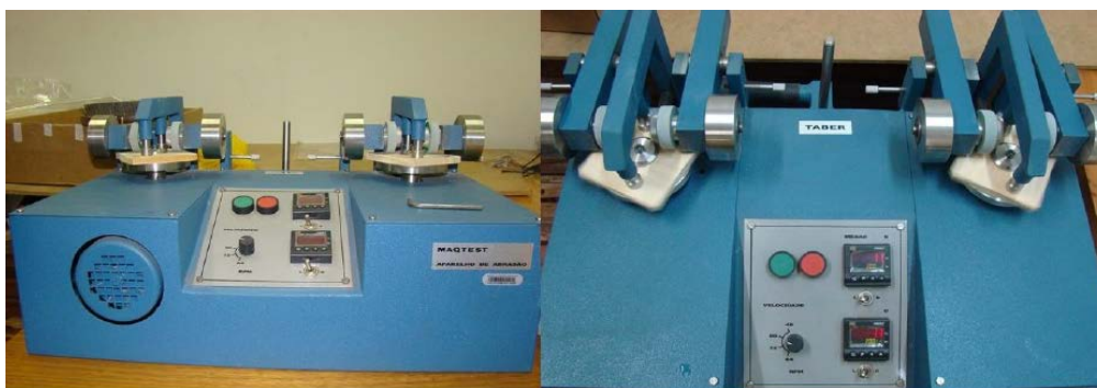
Fig. 1. Taber equipment used for the abrasion test.
