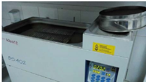
Fig. 2. NUVE-BS402 equipment used for the determination of the swelling in thickness after water immersion of the tested particleboards.
