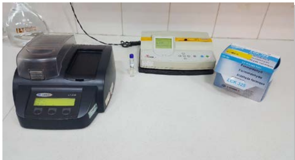
Fig. 1. Spectrophotometer for the determination of the formaldehyde emission by the flask method.
