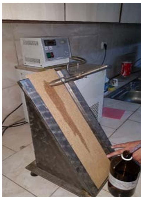
Fig. 3. Experimental set-up with inclined support and dropping pipette, for the determination of the surface absorption.
