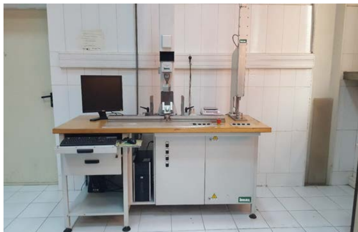
Fig. 4. IMAL IB600 equipment used for the determination of the mechanical properties of the tested particleboards.
