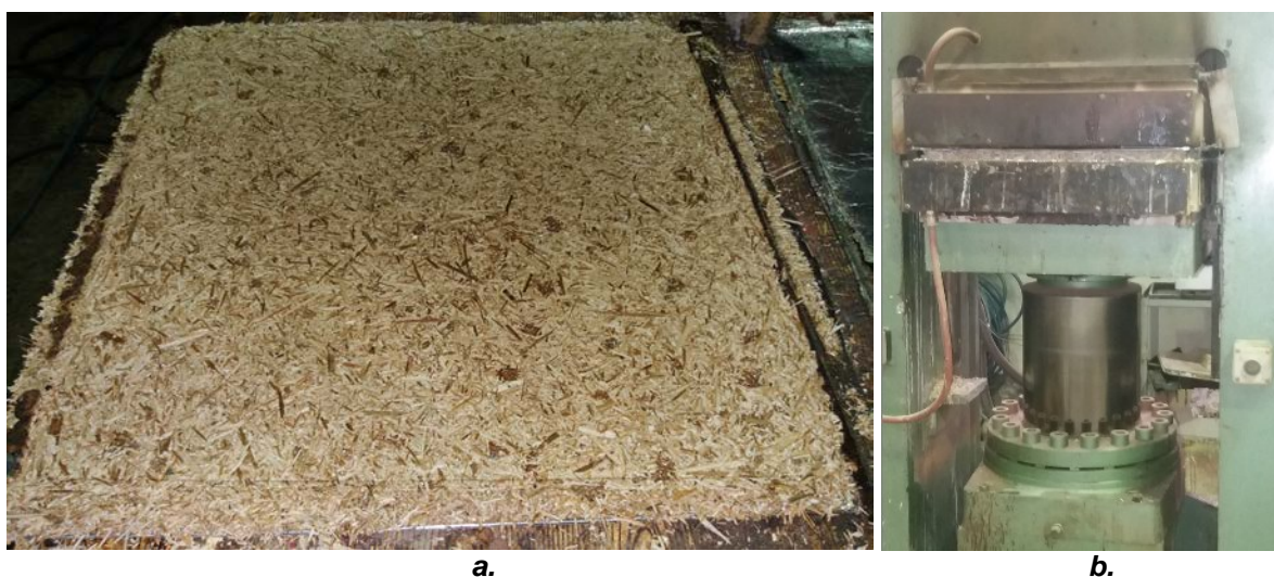
Fig. 3. Single layer particleboard (a) and press used to manufacture the boards (b).
