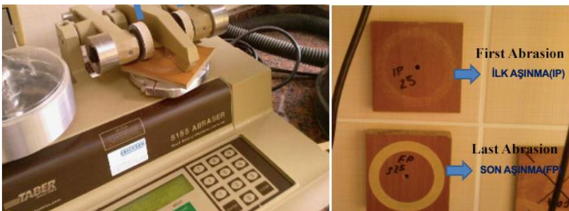
Fig. 2. Taber Abraser and tested samples.
