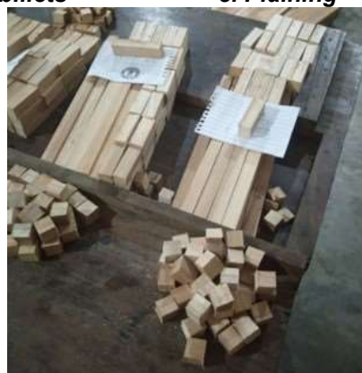
e. Converted to test samples of different dimensions
