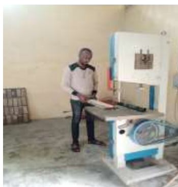
b. Converting planks to billets
