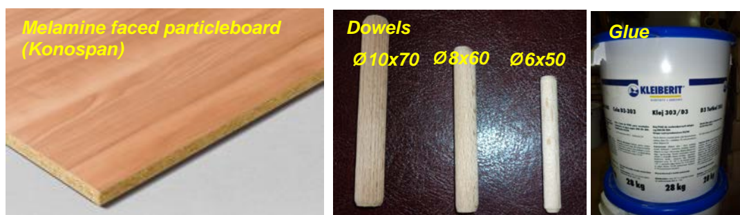
Fig. 1 Materials used for the dowel joints.
