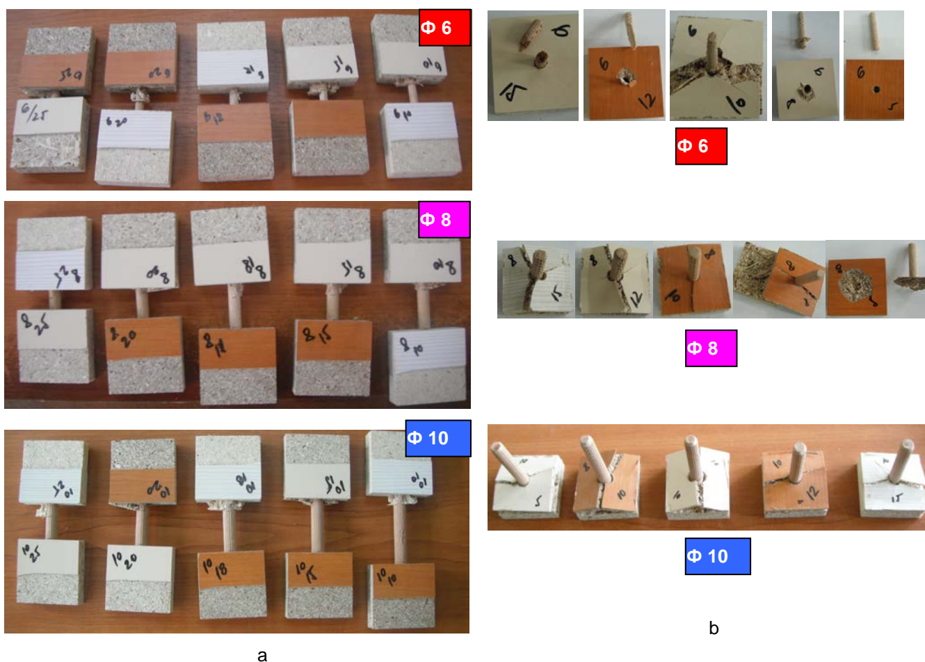
Fig. 9 Way of breaking the specimens; a – parallel tensile test; b – perpendicular tensile test.
