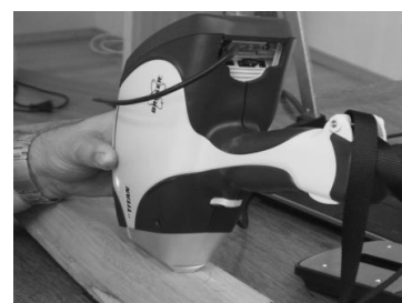
Fig. 6. XRF Analysis with S1 TITAN Series Handheld XRF Analyzer
