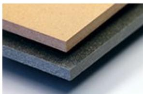
These boards are composed of around 60 percent wood particles and 40 percent thermoplastic material, generally polypropylene or polyethylene. Both wood and plastic components can be sourced from recycling streams. The wood component in WPC boards can be replaced by other lignocellulose products derived from the fibrous part of plants such as hemp or cotton, or the husks of rice grains and sunflower seeds. All of these materials are 100-percent recyclable.
