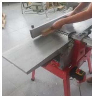
**b. Straightening, planing to thickness**
